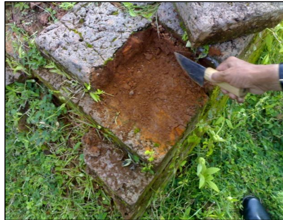
Fig 3: Collection of Mortar Sample
